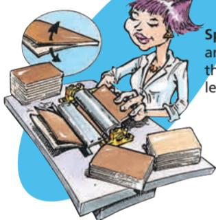
**Splitting** is vital to obtain the ideal thickness and to allow components to be put together in the best way possible. If necessary, each piece of leather is divided in two horizontally.
