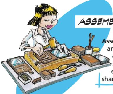
**Assembling** pre-glued pieces calls for accuracy and skill from the operator; it remains a **manual** operation. Once the pieces have been super-imposed, an **overcut tool** is used to eliminate any excess material and to obtain sharp edges.
