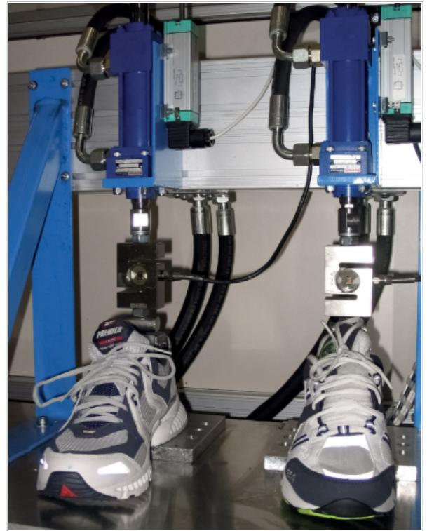
Type: [Physical and mechanical test](#)
